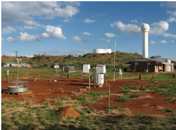
Figure 1. The weather station at Tennant Creek photographed on 17 January 2012 (BoM photograph from the ACORN-SAT catalogue). The louvered box or Stevenson screen (right of centre) houses thermometers and platinum resistance temperature probes installed in 1990 and used in their place by the automatic weather station (AWS) since 1996, at the standard height of 1.2m above the ground. The screen appears to be an older 230-litre type. Metadata indicates that manual thermometers and the galvanised A-pan evaporimeter on the left of the picture were removed on 1 June 2017.
