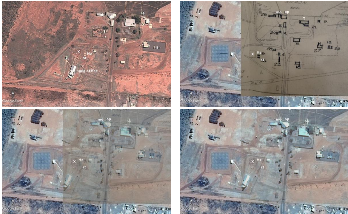
398 Figure 10. Google Earth Pro satellite image showing the 1969 met office and surrounds in September 2012 399 (upper left). Upper right, the image for March 2013 overlaid by a re-scaled 1950s aerodrome plan (100% 400 opacity) showing the location of the Aeradio office (mo), operations centre (op), terminal (T), H 2 shed for 401 preparing weather balloons (H 2 ) and met-store (ms) beside the instrument enclosure (x). Lower left is the same 402 image with the overlay map at 60% opacity and on the right, at 30%.
