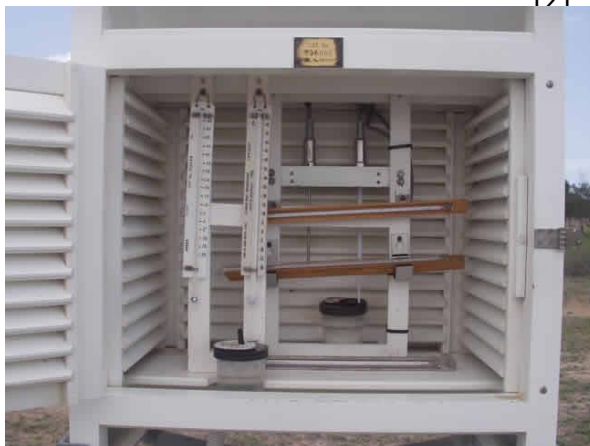
Figure 1. Inside the current 60-litre Stevenson screen at Townsville airport. At the front are dry and wet-bulb thermometers, behind are maximum (mercury) and minimum (alcohol) thermometers, held horizontally to minimise "wind-shake" which can re-set the instruments, and at the rear, which faces north, are dry and wet-bulb PRT (AWS) sensors. Moistened by a small patch of muslin tied by a cotton wick that dips into the water reservoir, dry-bulb minus wet-bulb T (wet-bulb depression) is used to estimate relative humidity and dew point temperature. (BoM photograph).
