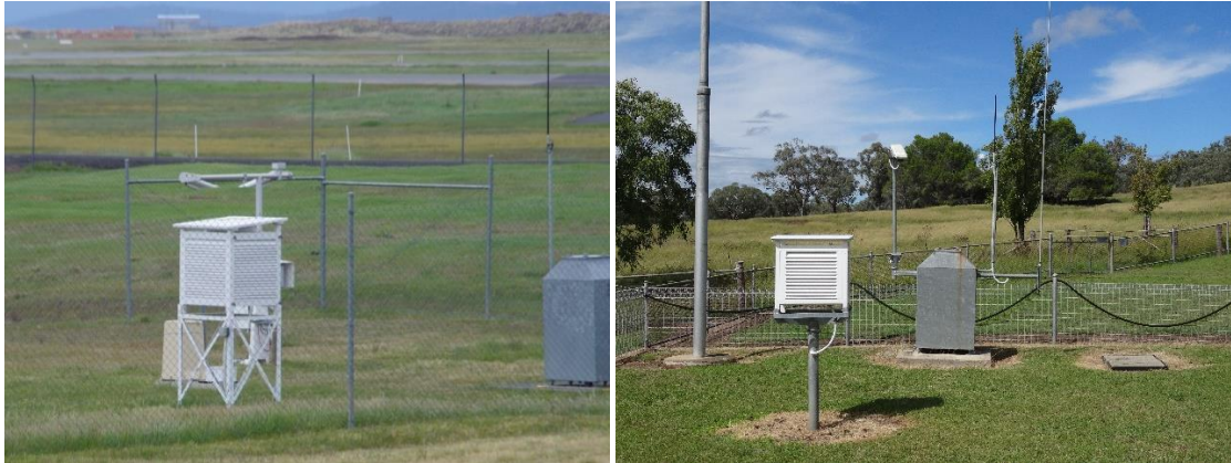
341 Figure 6. The large (230-litre) Stevenson screen at Hobart airport behind a 2.2 m Cyclone fence 342 photographed from a distance by the Author on 20 October 2016; and right, the small (60-litre) screen at 343 Inverell Research Station photographed on 15 March 2017.
