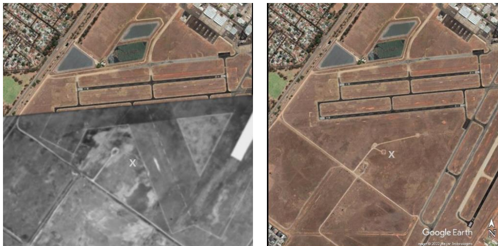
82 Figure 2. A rescaled overlay of a portion of the greyscale November 1968 South Australian Government aerial 83 photograph and a Google Earth Pro satellite image for February 2019. Meteorological instruments are 84 identifiable in both images immediately left of the point marked 'x'. Note the airport was redesigned from its 85 earlier 'A' configuration to parallel and offset runways and taxiways in the 1970s.
