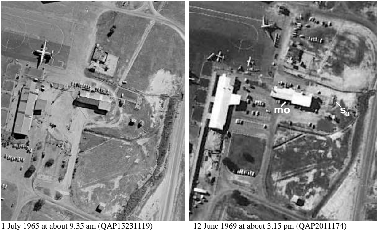
Figure 8. Aerial photographs show the met-office was extended between July 1965 and June 1969. A memo in the Garbutt instrument file (p. 70; 29 October 1969) notes that extensions to the building “restricts the sun reaching the (sunshine recorder and actinograph) from 5 pm”.
