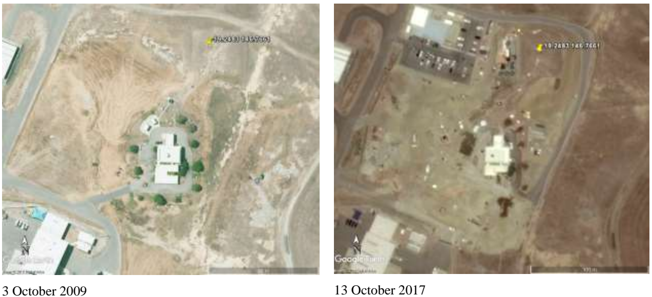
Figure 9. Google Earth Pro satellite images show developments in the vicinity of the Townsville airport met-enclosure are permanent and likely to impact on temperature measurements. Google Earth Pro measurement tools show hardstand areas to the west of the site are within 17 m of the Stevenson screen.
