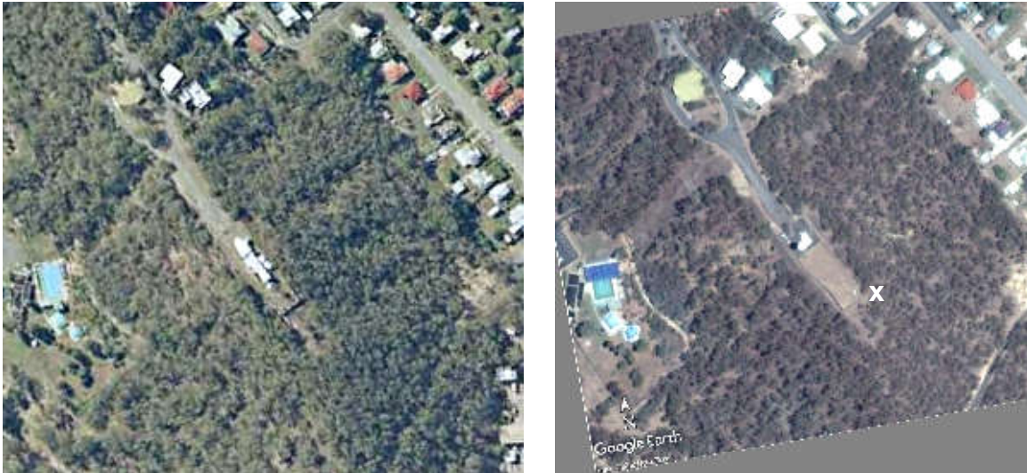
Figure 1. The Gladstone Radar met-office on 17 May 2003 (left; portion of QAP5850057) and 4 January 2006 (Google Earth Pro satellite image). The Stevenson screen and AWS cabinet visible in the satellite image near (x) was relocated from behind the office during the intervening period. Images are comparably scaled and aligned. Trees up to 6 m in height surround the cleared area. The site was reconfigured when the office was demolished in 2004.
